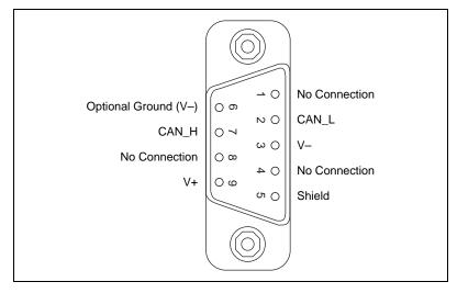
Figure B-1. Pinout for 9-Pin D-Sub Connector
